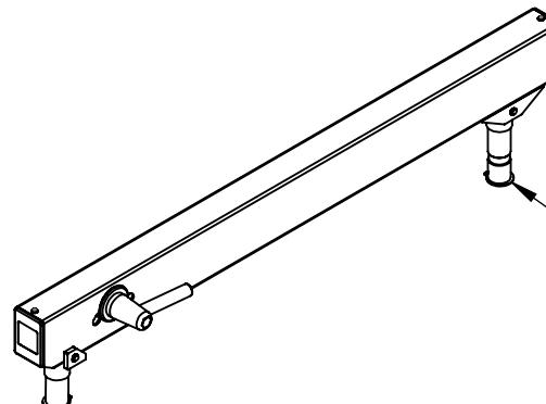
**2X REMOVEABLE EXTERNAL RETAINING RINGS
