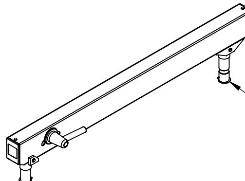
**2X REMOVEABLE EXTERNAL RETAINING RINGS TO SECURE ASSEMBLIES**
