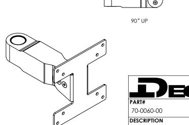
QTY. (4) M4 x 0.7 x 10MM Phillips Drive Button Head Screws included in package will inteface with most standard monitors featuring VESA hole configuration. Please reference your monitors manual for suggested monitor mounting hardware.
